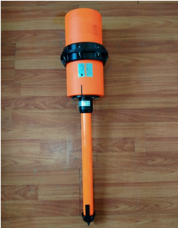
Gambar 4.2 Unit antenna RT-400
