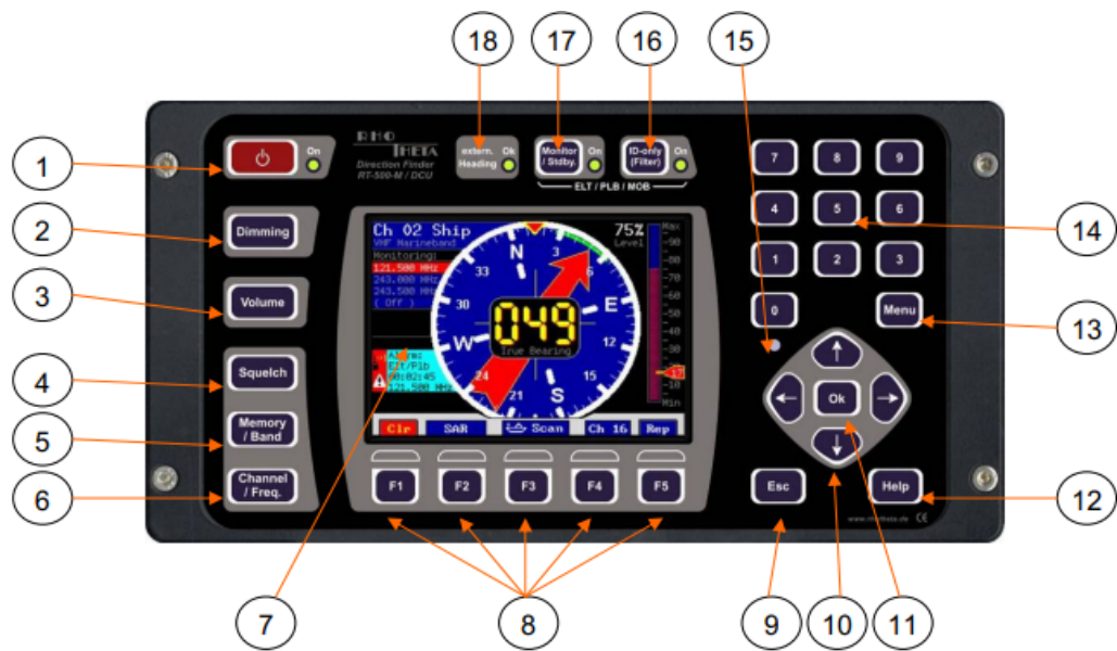
Gambar 3.3 Fitur-fitur fisik display control unit Rhotheta RT-500
